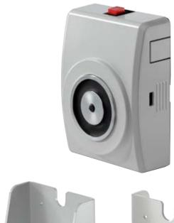
The Zeta magnetic door holders are designed to retain a fire door open against the force of its own closing device. In the event of a fire, the door holder magnet can be turned off by the fire alarm, allowing the door to shut.
