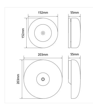
The Zeta motorised fire alarm bells combine styling and functional efficiency. They incorporate a low power rotary centrifugal mechanism, which gives a high sound output with low current consumption at 24V dc.
